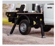
Double A-frame outriggers front and rear for compact setup
