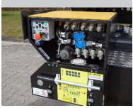
Emergency ground controls located within a seperate compartment.
