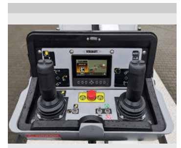
XPC controls: Variable outreach (with load cell) and up to 4 actions at a time
