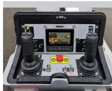
XPC controls with up to 4 actions at a time & automatic outrigger setup and packing
