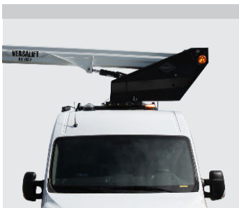
Turret/knuckle tail swing and outriggers within the mirrors
