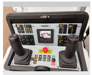
LMC (Load Moment Controls): Variable outreach and up to 2 actions at a time (1 per joystick)
